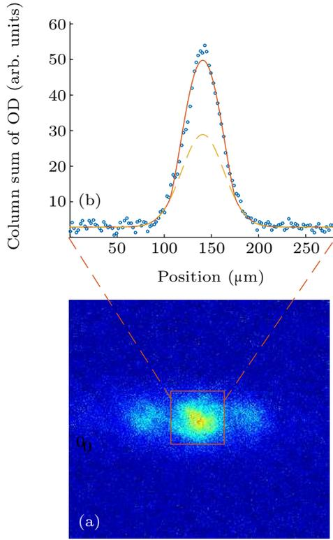
**Fig. 2.** (a) Interference pattern of the Bose–Einstein condensate released from a 1D optical lattice of the depth  $V_0 = 2.4E_r$  after a time of flight of 7 ms. (b) The fit (solid line) and the column sum of the optical density (OD) (circles). The dashed line is the Gaussian fitting for the distribution of thermal gas.
