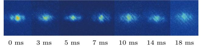
**Fig. 4.** Interference pattern of a Bose–Einstein condensate released from a 1D optical lattice of depth  $V_0 = 2.4E_r$  with various holding time after a time of flight of 7 ms.
