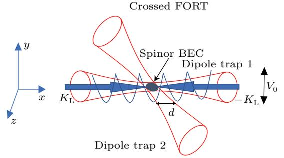
**Fig. 1.** Schematic setup of the experiment. A 1D lattice potential is formed by overlapping an optical standing wave along the horizontal axis ( $x$  axis) with a Bose-Einstein condensate in a crossed dipole trap. The parameters  $V_0$  is the lattice depth and  $d$  is the lattice spacing.
