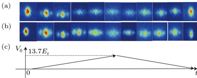
**Fig. 3.** (a) and (b) Observation of the superfluid to Mott insulator transition: The lattice depths for the sequence of images from left to right are (0, 2.4, 5.5, 8.2, 11, 13.7, 11, 8.2, 5.5, 2.4, 0)  $E_r$ . (c) Time dependence of the lattice depth. For Fig. 3(a), the time step is 3 ms for each depth, while for Fig. 3(b), it is 2 ms. The total ramp time is 30 ms and 20 ms.
