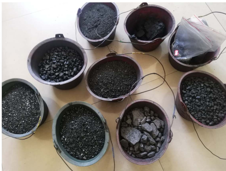
(a) Some of the original samples of clean coal, medium coal, slime and gangue were collected.
