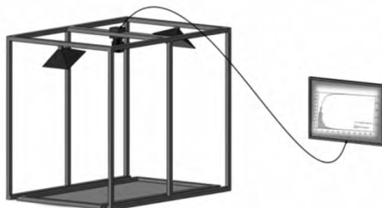
Fig. 1 Schematic of the experimental set-up for coal gangue particle size distribution analysis
